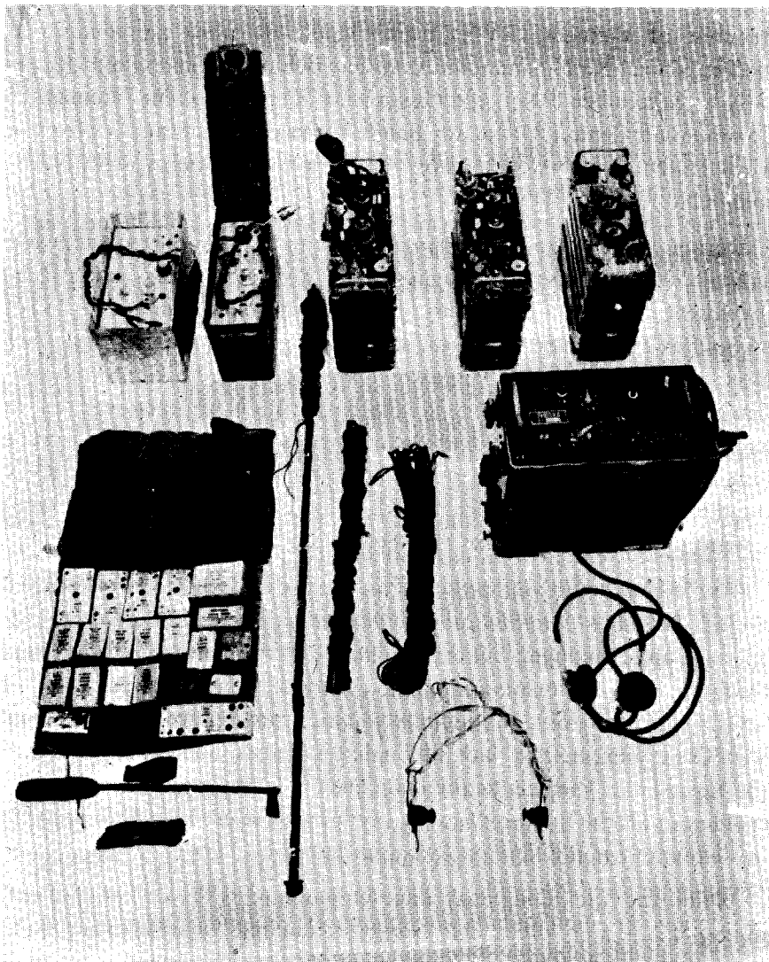
Communications Equipment Captured From an Enemy SIGINT Unit. (Top, left to right: a homemade transmitter, a homemade receiver, two U.S. AN/PRC-25's, and a U.S. AN/PRC-77. Bottom, left to right: radio receiver parts, antenna parts, wire, headphone, and a CHICOM R-139 receiver with headphone.)
